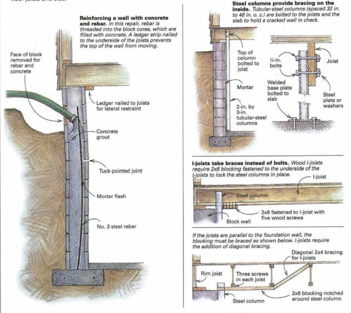
The first method-filling the core with rebar and concrete—requires removing the exterior faces of concrete blocks near the grade line (not at the top), inserting #3 steel rebar into the block cores and pushing it down to the footing (drawing above). This can be done in every core or as much as 48 in. apart (I have seen it done both ways). The cores are then filled with a concrete slurry mix.
